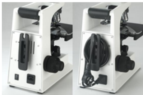
Wire winding device convenient for carry and storage
